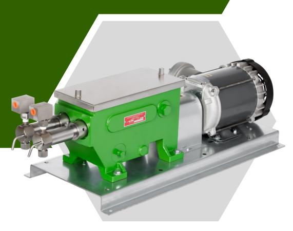
The model MT chemical injection pumps are designed to be driven by an electric motor. These positive displacement pumps have removable fluid ends with interchangeable check valves, and a removable stainless steel cover for easy maintenance on the drivetrain.
