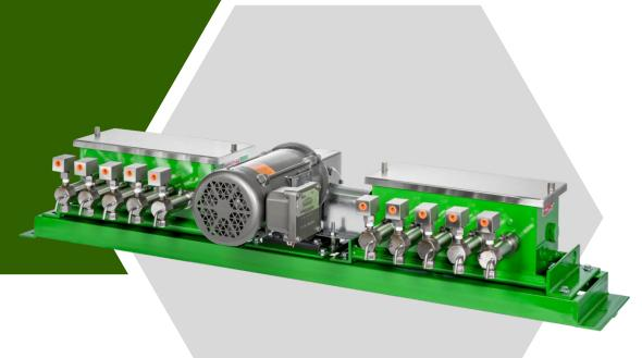
The model MH chemical injection pumps are designed to be driven by an electric motor. These positive displacement pumps have removable fluid ends with interchangeable check valves, and a removable stainless steel cover for easy maintenance on the drivetrain.
