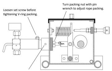
Turn fluid end nut with pin wrench to adjust V-ring packing.
