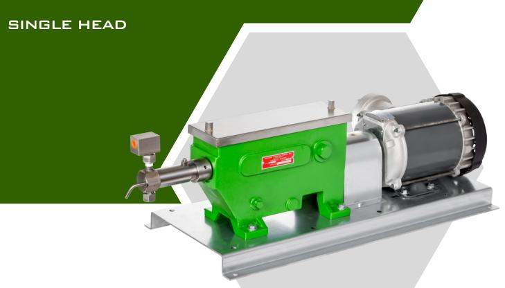
The model MA chemical injection pumps are designed to be driven by an electric motor. These positive displacement pumps have removable fluid ends with interchangeable check valves, and a removable stainless steel cover for easy maintenance on the drivetrain.
